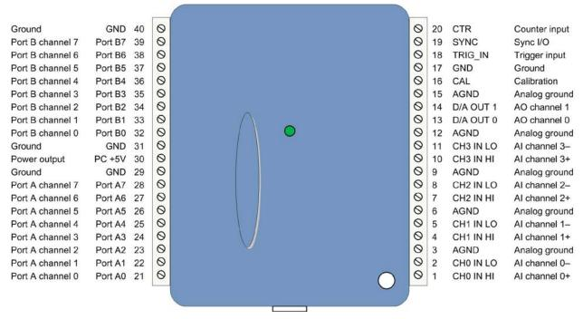
Figure 4. Differential mode pinout
