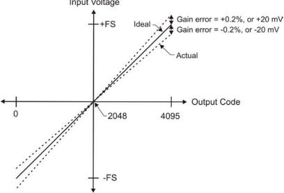
Figure 13. ADC Transfer function with gain error
