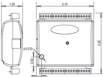
Figure 15. Circuit board (top) and enclosure dimensions
