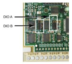
Figure 9. Pull-up/down jumper locations
