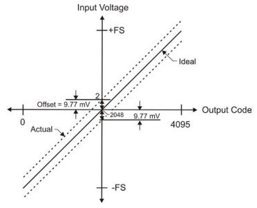
Figure 12. ADC transfer function with offset error
