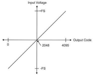
Figure 11. Ideal ADC transfer function
