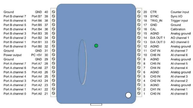
Figure 3. Single-ended mode pinout
