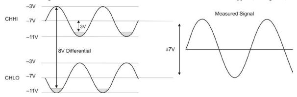
Figure 7. Differential voltage example: common mode voltage of -7 V
