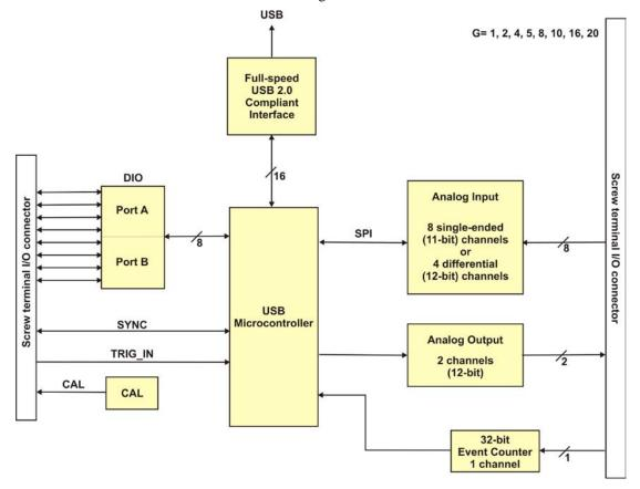
Figure 1. USB-1208FS functional block diagram
