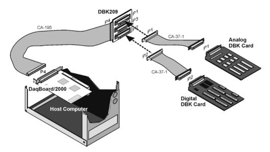
Using a DBK209 to Connect an Analog and a Digital DBK Card to DaqBoard/2000
