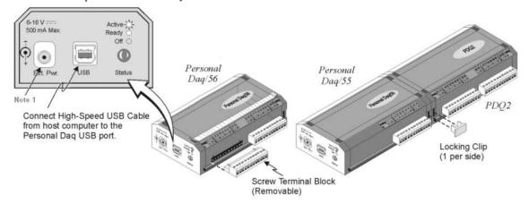
**Note 1**: Typically, there is no need to connect power to the External Power connecter. Most PC USB ports supply the needed 500 mA at 4 to 5.25 V. However, some notebooks do not. In such cases, the Personal Daq unit will require the use of a power adapter.
