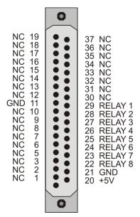
Use C37FF-x cables to connect with compatible MCC 24-bit digital I/O boards, such as the USB-DIO24/37. The 2<sup>nd</sup> connector is provided to access the remaining board connections.
