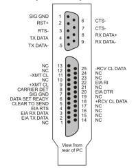
The **CIO-COM422** combines an RS232 and an RS422 interface with a single communications port. RS232 is commonly a 25-pin connector, while RS422 is a 9-pin connector.
