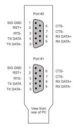
The **CIO-DUAL422** combines a pair of communications ports each with RS422 standard interfaces. Each COM port uses one of the 9-pin connectors shown here.
