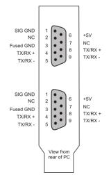
The CIO-COM485 is equipped with two DB9 connectors for RS485 standard 9-pin connectors and cables. The RS485 standard allows multiple transmitters and receivers on a single communications cable.
