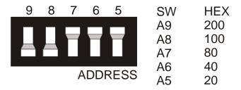
Figure 1. Base address switch
