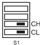
Figure 6. Switch S1 default configuration
