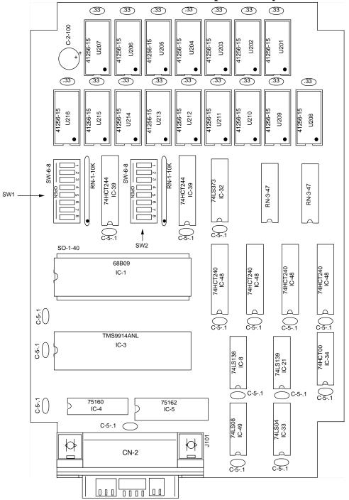
6.10 Serial488/512K I/O Board Component Layout
