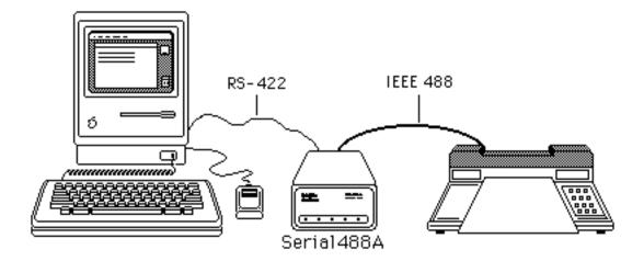
The Macintosh computer outputs RS-422 levels. Because of this, the internal DIP shorting jumper is set to the RS-422 position (J205).
