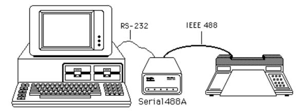
The following shows the **Serial488A**'s internal switch settings required to use a Hewlett Packard 7580A plotter with AutoCad<sup>TM</sup> from AutoDesk on an IBM PC or compatible. Because PC and compatibles output RS-232 levels, the shorting DIP jumper should be set to the RS-232 position (J206).
