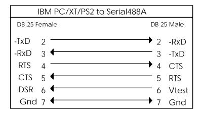
IBM PC/XT/PS2 to Serial488A Wiring Diagram (RS-232)
