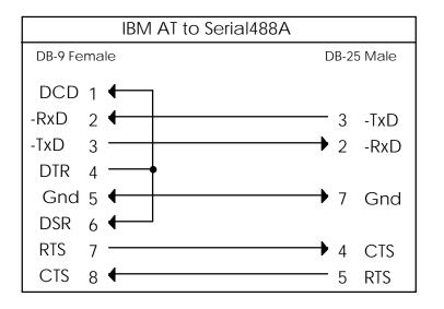
Note: Standard AT 9 Pin to 25 Pin adapter cables are not wired as shown above and will not work with the **Serial488A**.
