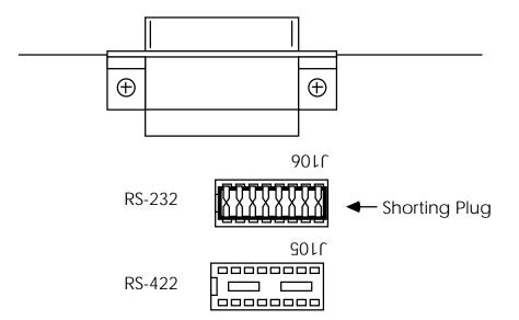
Selecting RS-232 Signal Levels - Serial488A/OEM
