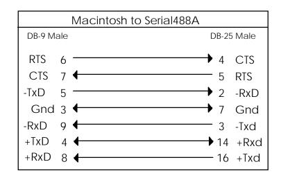
Macintosh to Serial488A Wiring Diagram (RS-422)
