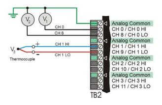
To differentially connect a thermocouple; connect the red T/C wire to the channel's Low (L) connector. Connect the *other color* wire to the channel's High (H) connector.
