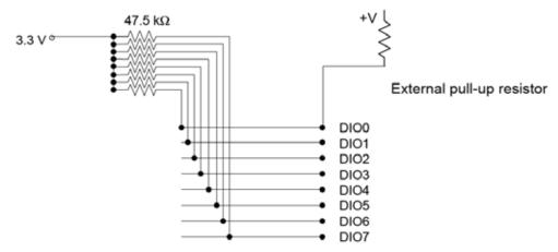
Figure 4. Digital I/O external resistor configuration
