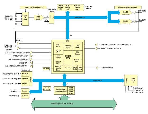
Figure 1-1. PCI-DAS6402/16 functional block diagram
