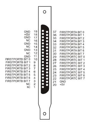
Figure 2-5. BP40-37 cable pin out
