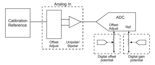
Figure 4-1. Analog input calibration
