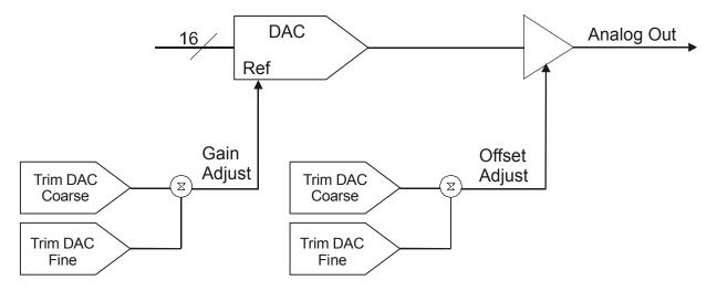
Figure 4-2. Analog output calibration
