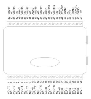
Figure 5. USB-3114 signal pin out
