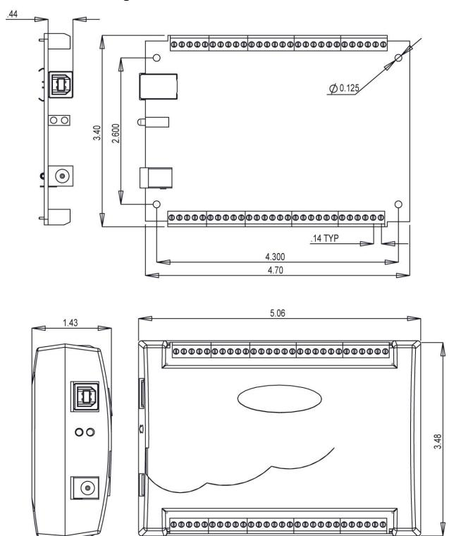
Figure 9. Circuit board (top) and housing dimensions
