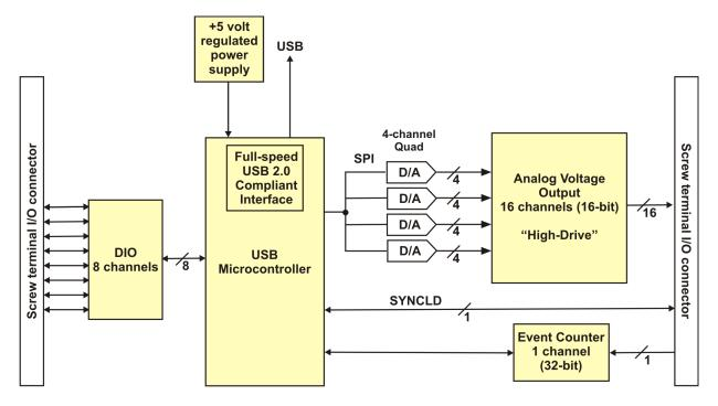
Figure 2. USB-3114 block diagram
