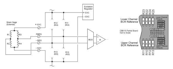
Full Bridge, Resistor Configuration for DBK16
