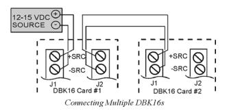
The user-supplied excitation source is attached to a voltage regulator in the DBK16 circuitry. This regulator provides the excitation to the actual transducer (there is a separate regulator for each transducer, hence two regulators per DBK16). Each regulator has a maximum current of  $50 \, \text{mA}$ . The maximum amount of excitation that can be provided by the DBK16 excitation regulator is represented by the following equation:
