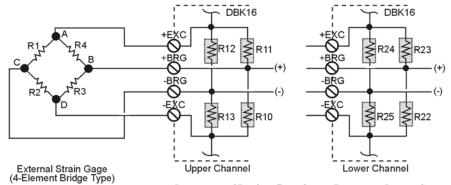
Locations of Bridge-Completion Resistors (Internal)
