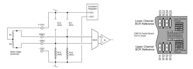
*Half Bridge*, ( $\Delta R1 \downarrow \text{ and } \Delta R2 \uparrow) \Rightarrow \Delta E_{OUT} \uparrow$ ) *Resistor Configuration for DBK16*
