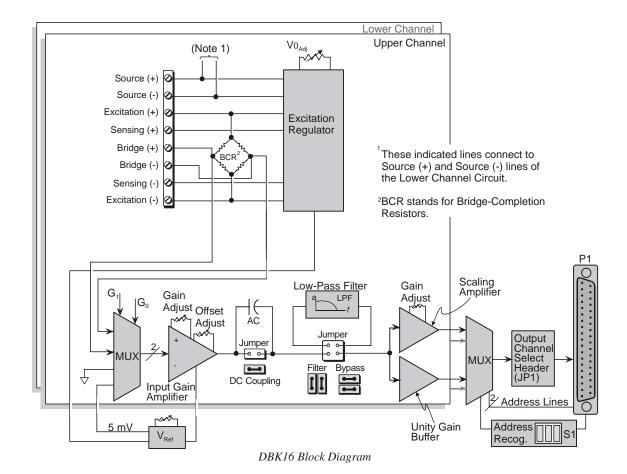
A wide-range excitation regulator is adjustable from 1.5 to 10.5 VDC with a current limit of 50 mA. The DBK16 requires a 12 to 15 VDC external excitation voltage that can be supplied from the DBK30A battery module or other user-supplied source.
