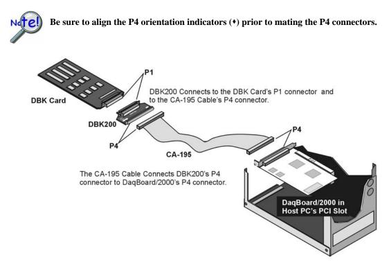
Connecting a DBK Card to a DaqBoard/2000 Series Board via a DBK200
