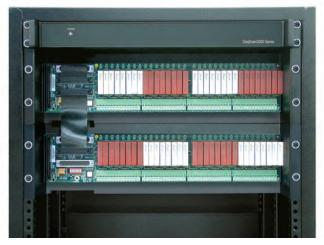
The 64-channel isolated discrete I/O system consists of one DaqScan plus two DBK210 boards with rack-mount kits
