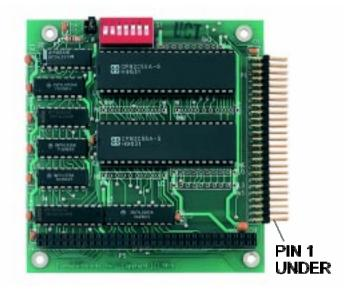
Figure 2-2. PC104-DIO48 Board Layout and Pin 1 Location
