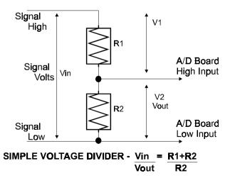
Figure 5-2. Voltage Divider
