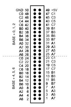
Figure 2-2 I/O Connector
