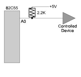
Figure 5-1. Output Being Pulled Up
