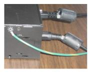
This partial view of the data acquisition device shows its connection to the ground-line. It also shows two ferrite collars, the foremost of which is clamped to the power cable. The background collar is clamped onto the Ethernet cable.
