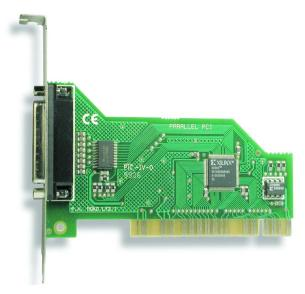
The WBK23 PCI/EPP Interface Plug-In Board
