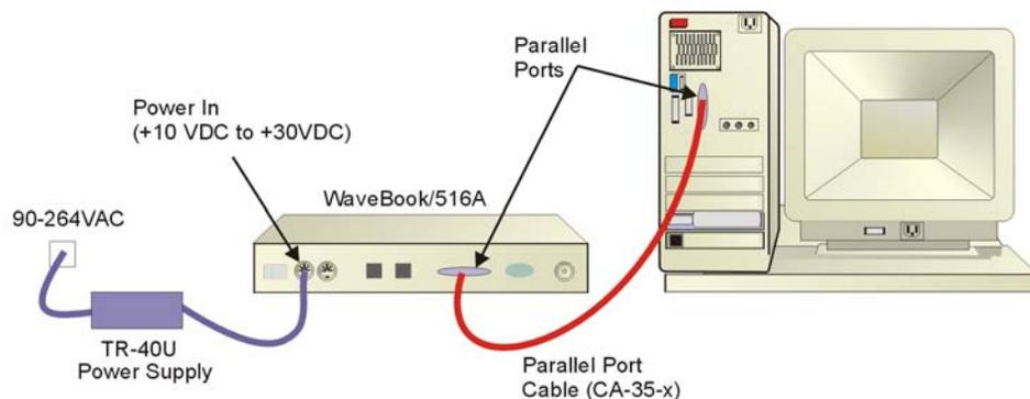
1. Using a parallel port cable, connect the WaveBook to a parallel port on the computer.
