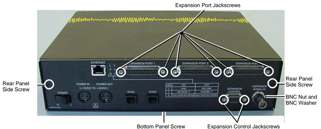
7. Remove the Rear Panel from the main chassis (see following figure).
