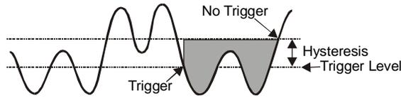
This trigger is the reverse of the rising-edge trigger: the trigger becomes valid after the signal level has been above the hysteresis range and then goes below the trigger level. This trigger becomes invalid whenever the signal level goes above the hysteresis range. This prevents the false triggering that would occur with below-level triggering if the signal was below the trigger level at the start of the acquisition.
