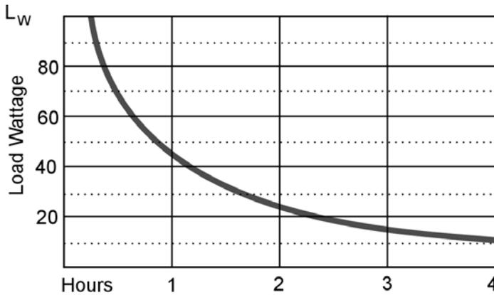
Graph indicates approximate battery life under the indicated Load Wattage @ 25°C (77°F).
