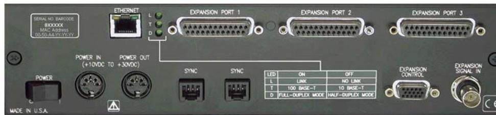
**MAC Address Label:** The Media Access Control (MAC) label is located in the upper left corner of the rear panel. The label shows the device serial number in barcode and base 10 formats. It also shows the Ethernet address (MAC Address) which is derived from the serial number in hexadecimal. If prompted to enter a serial number in software, use the base 10 number. Conversion to a hexadecimal number for use in addressing will be automatic.
