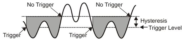
This trigger is valid whenever the signal level is below the trigger level and stays valid until the signal level goes above the hysteresis range (the reverse of above-level triggering). As with all multi-channel trigger types, WaveBook's actual trigger depends on the combination of this trigger with the other channels' trigger states.
