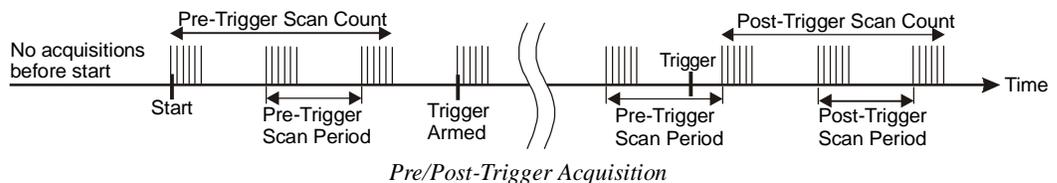
The time needed to complete the final pre-trigger scan is part of the trigger latency; and so, in the pre/post-trigger mode, the trigger latency may be greatly increased.
