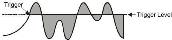
In this trigger type, the channel becomes valid when the signal level rises above the trigger level and stays valid until the acquisition is complete and WaveBook is re-armed.
