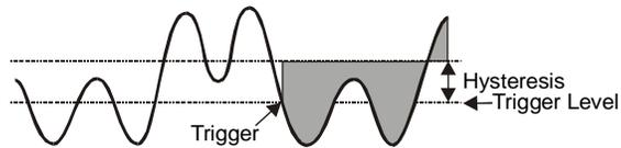
This trigger is the reverse of the rising-edge-with-latch trigger: the trigger becomes valid after the signal level has been above the hysteresis range and then goes below the trigger level. The trigger remains valid until the acquisition is complete.
