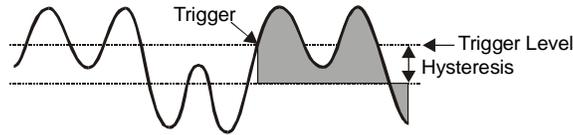
This trigger becomes valid like a rising-edge trigger: when the signal level goes above the trigger level after first being below the trigger range. However, the rising-edge-with-latch trigger does not become invalid, regardless of the signal level, until the acquisition is complete. Rising-edge-with-latch is used to trigger after the channel has reached the trigger level, rather than just while the channel is above the trigger level.
