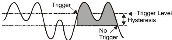
This trigger becomes valid after the signal level has been below the hysteresis range and then goes above the trigger level. This trigger becomes invalid when the signal level goes below the hysteresis range. Unlike above-level triggering, the channel cannot become valid until the signal level first goes below the hysteresis range. This prevents the false triggering that would occur if the signal were above the trigger level at the start of the acquisition.
