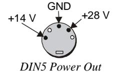
The CA-115 cable connects to DBK30A's POWER OUT connector and WaveBook's POWER IN connector. The cable can be used to daisy-chain a DBK30A unit to a WBK expansion module.
