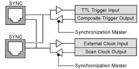
The above diagram shows how an “A” or “E” Series WaveBook can input or output synchronization timing and trigger events on either SYNC connector. A more detailed block diagram follows.
