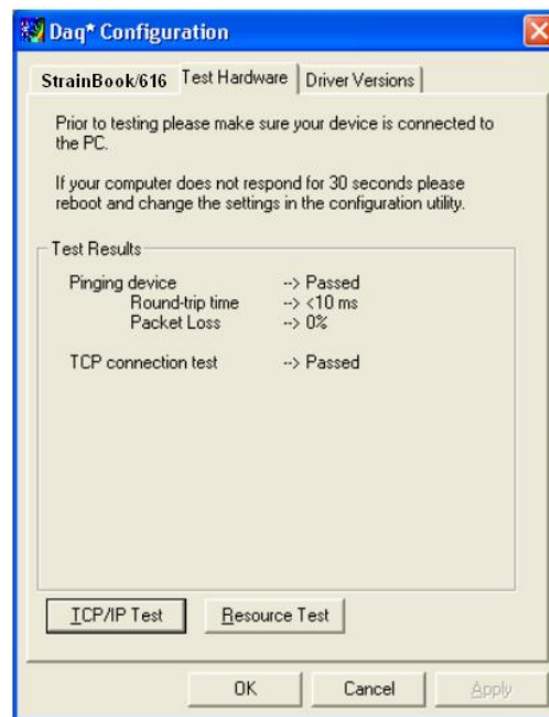
Results of a TCP/IP Test for a StrainBook/616
