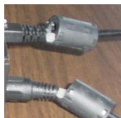
A view of two ferrite collars close to StrainBook's rear panel. The closest is clamped to the power cable. The background collar is clamped to the Ethernet cable.
