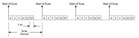
Notice that some of the analog channels in the scan group are from a PDQ30 expansion module. All analog channels are sampled at the same rate of 1us. Analog channels on the PDQ30 can also have any of the gain ranges applied.
