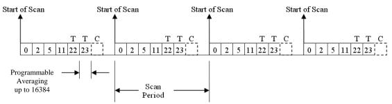
In this example, the desired number of oversamples is 256, therefore each analog channel in the scan group requires 256 microseconds to return one 16-bit value. The oversampling is also done for CJC temperature measurement channels. The minimum scan period for this example is therefore 7 X 256  $\mu$ s, or 1792 microseconds. The maximum scan frequency is the inverse of this number, 558 Hz.
