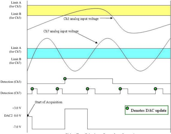
Using Two Criteria to Control an Output\*
