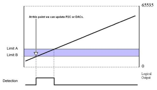
Channel 1 in Totalizing Counter Mode, Inside the Window Setpoint
