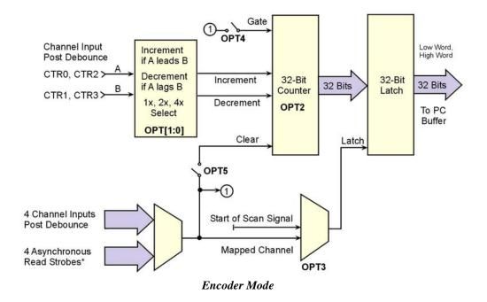
\*There is one asynchronous read strobe for each of the four counter channels.
