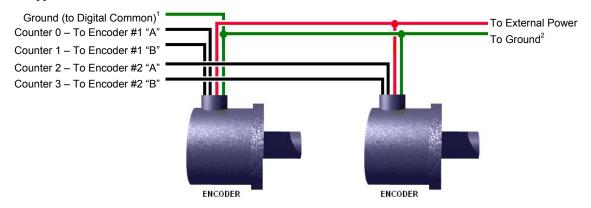
Two Encoders Connected to Personal Daq/3000
