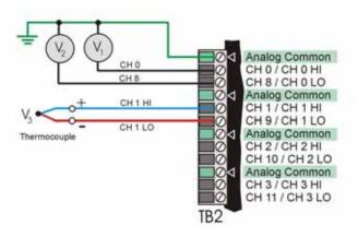
Single-Ended (V1 and V2) and Differential (V3) Connections to Analog Input Channels
