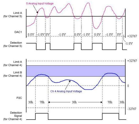
Analog Inputs with Setpoints Update on True and False In the example [upper portion of the preceding figure], the setpoint placed on analog Channel 5 updated DAC1 with 0.0V. The update occurred when Channel 5's input was less than the setpoint (Limit A). When the value of Channel 5's input was above setpoint Limit A, the condition of <A was false and DAC1 was then updated with *minus*1.0V.
