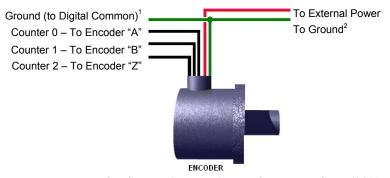
*Encoder Connections to pins on the Personal Daq/3000* <sup>1</sup>The ground depicted at the left is associated with Digital Common on the Personal Daq/3000 Series module. <sup>2</sup>The ground depicted at the right is associated with the external power source.
