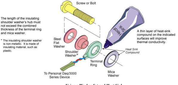
Using a Washer Set and Heat Sink to Isolate the Thermocouple
