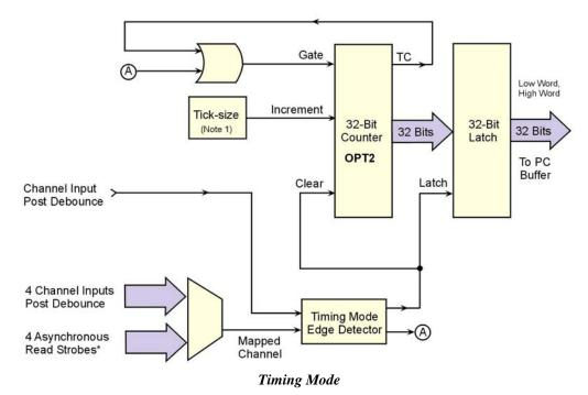
\*There is one asynchronous read strobe for each of the four counter channels.
