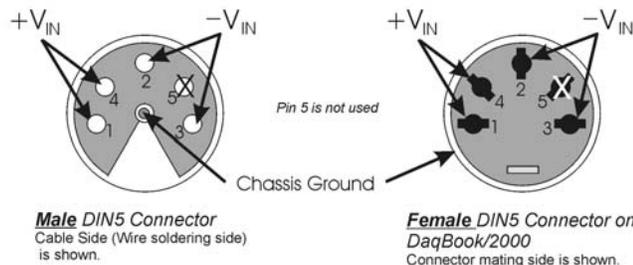
The lines that will connect to the vehicle battery are soldered to the male DIN5 connector. As indicated in the first figure on this page, the  $+V_{IN}$  line connects to the battery's positive (+) terminal and should have a 7.5 amp fuse in series with the line. The  $-V_{IN}$  and Chassis Ground lines both connect to the battery's negative terminal.
