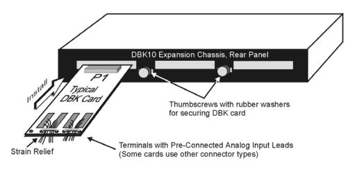
Installing a Card in a DBK10 Expansion Chassis
