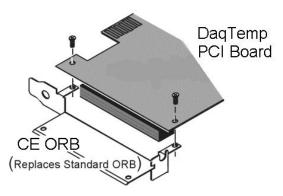
Mounting a DaqTemp Series PCI Board to a CE ORB
