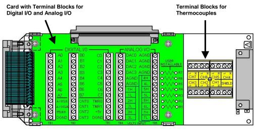
DaqTemp7A and DaqTemp7, Internal Layout
