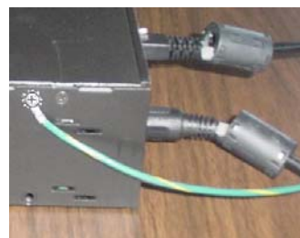
This partial view of the data acquisition device shows its connection to the ground-line. It also shows two ferrite collars, the foremost of which is clamped to the power cable. The background collar is clamped onto the Ethernet cable.
