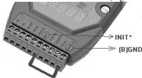
Figure 2-21. Shorting “INIT*” and “(B) GND”.
