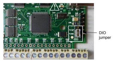
Figure 5. Pull-up/down jumper location
