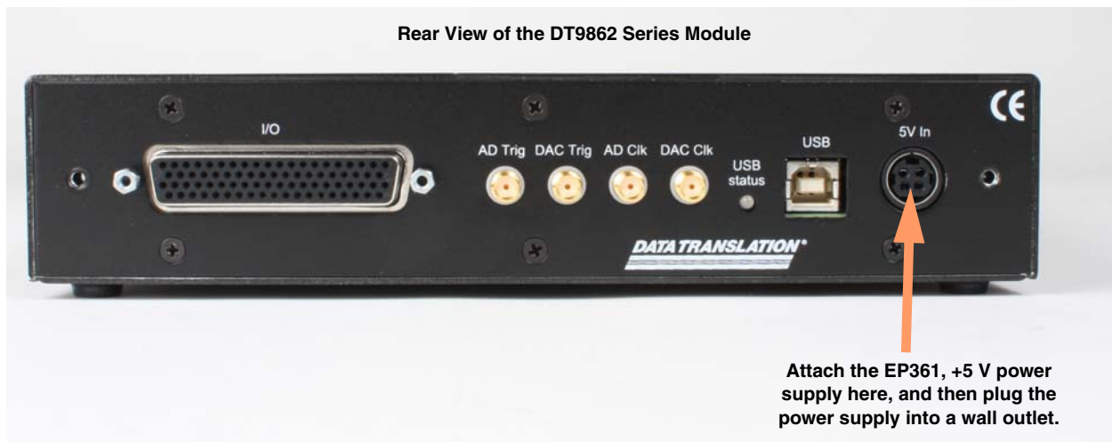
Figure 3: Attaching a +5 V Power Supply to the DT9862 Series Module
