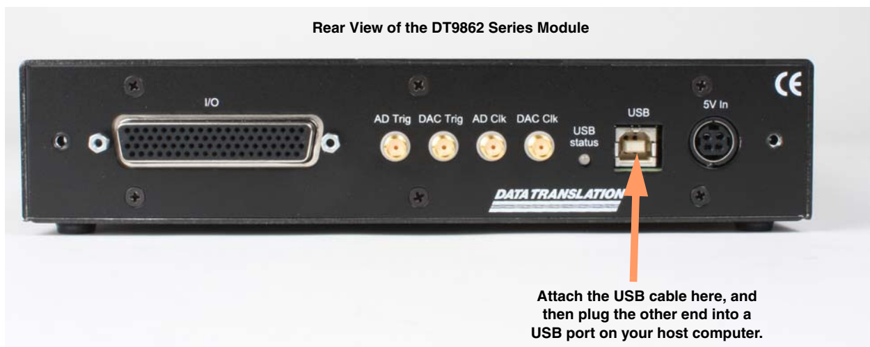
Figure 4: Attaching the USB Cable to the DT9862 Series Module
