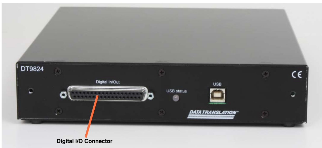
Figure 6: Digital I/O Connector of the DT9824 (Rear Panel)
