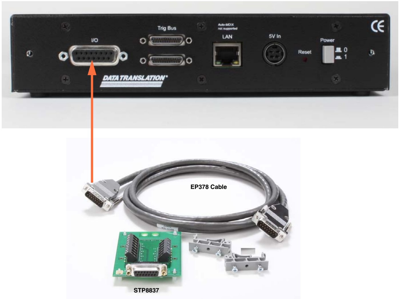
Figure 15: Connecting the DT8824 or DT8824-HV to the STP8837
