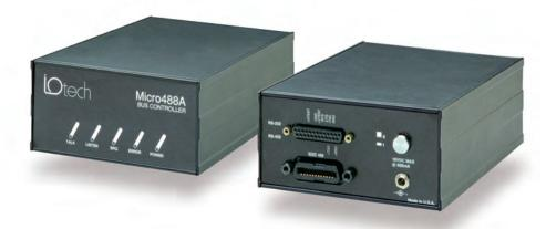
Micro488A converts any computer with a serial port into a full-featured IEEE controller
