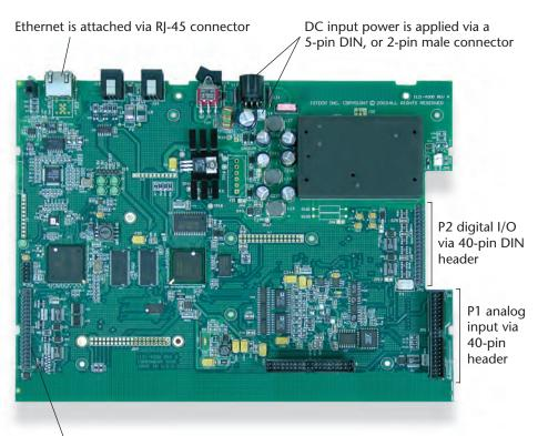
P3 frequency I/O, digital I/O, and optional analog output via 40-pin header
