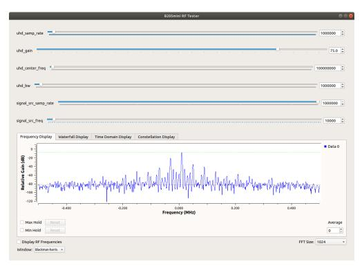
The UHD gain is the only exception. By default, as a hardware protection effort, the gain is set to zero. This RF signal strength from the b205mini will not be enough to make it through the attenuator and RF cabling for the ADP5250 to distinguish from the noise floor. Use the slider bar to increase the gain until the signal is visible on the spectrum analyzer of the ADP5250. The recommended gain values are 70dB - 90dB(max).
