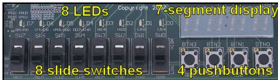
Figure 7: Nexys2 board I/O devices
