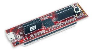
Microchip<sup>®</sup> PIC32MX150F128D microcontroller (40/50 Mhz 32-bit MIPS, 128K Flash, 32K SRAM)
