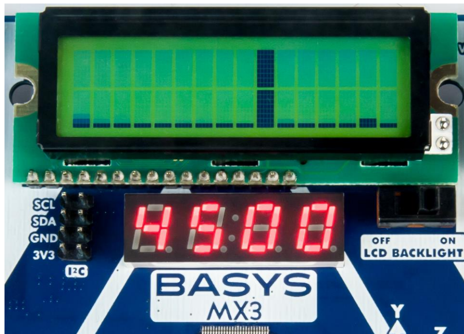
Figure 8.2. LCD and 7-segment display for spectrum analyzer.
