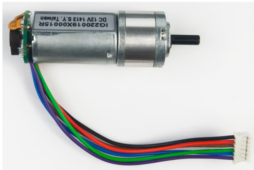
Figure 7.2. DC Motor with digital tachometer.
