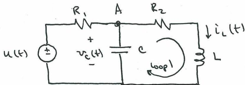
$$\text{KCL at } A: \frac{u - v_c}{R_1} = C \frac{dv_c}{dt} + i_L \quad (1)$$
