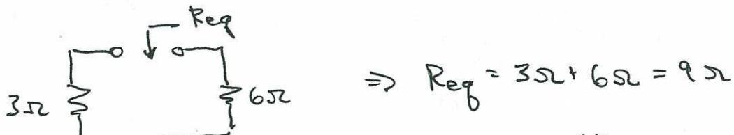
$$\Rightarrow R_{eq} = 3\Omega + 6\Omega = 9\Omega$$
