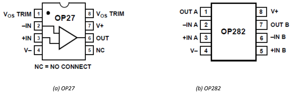
Figure 5.11. Additional operational amplifier pin connection examples.
