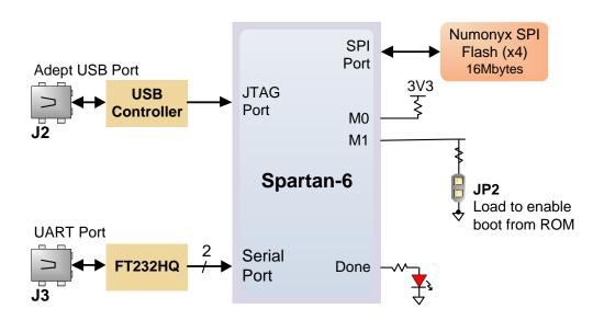
An on-board mode jumper (JP2) selects between JTAG/USB and ROM programming modes. If JP2 is loaded, the FPGA will automatically configure itself from the ROM. If JP2 is not loaded, the FPGA will remain idle after power-on until configured from the JTAG port.
