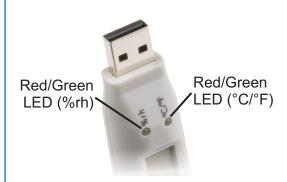
One LED is for temperature measurement, the other is for RH. The status indication alternates every 10 seconds. So, first you will see the status of the temperature logging; 10 seconds later you will see the status of the RH logging, and so on.
