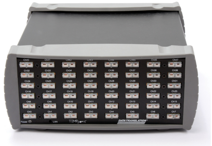
Figure 1. TEMPpoint allows direct connection of thermocouple, RTD, and voltage sensors with 1000V isolation between any of the 48 channels. Ground loops are eliminated through the isolation of each channel using the ISO-Channel technology.
