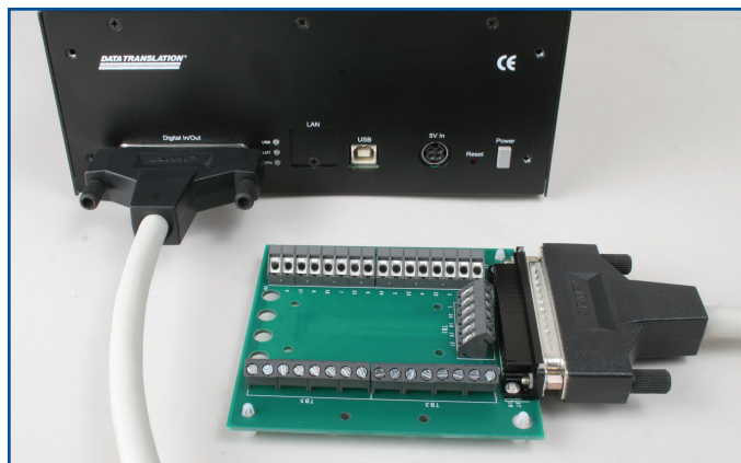
Figure 5. Digital inputs and outputs are easily connected via the 37-pin D-sub connector on the back of the instrument using the STP-37 screw terminal panel and 37-pin EP333 cable.
