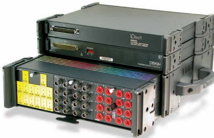
An assembled system consisting of a LogBook/360 plus a DBK84 thermocouple option, and a DBK50 isolated voltage input option
