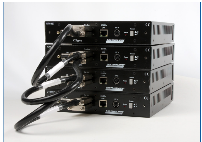
Up to 16 modules can be used in parallel to connect up to 64 direct voltage or IEPE channels, each synchronized in a master/slave configuration. The picture above shows four instrument modules in such a configuration.
