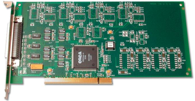
The DT335 features 32 digital I/O lines and interrupt on change.
