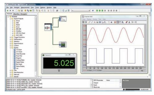
DASYLab lets you interactively develop PC-based data acquisition applications by simply attaching functional icons. DASYLab offers real-time analysis, control, and the ability to create custom graphical user interfaces (GUIs). What's more, in contrast to other graphical programming environments, which can require weeks of training to master, DASYLab has a very short user-learning curve. Many applications can be configured in a few minutes, rather than days or weeks.
