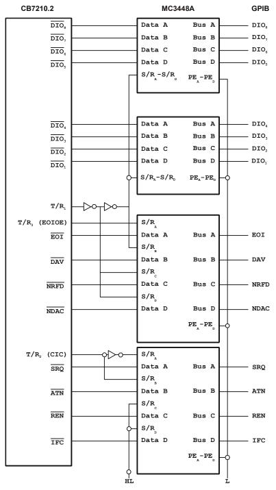
In this example, a high-speed transfer cannot be made, since the bus transceiver is an open collector type.
