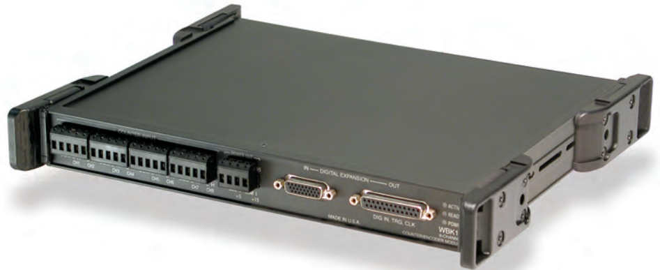
The WBK17 provides eight channels of 32-bit general-purpose counters, and is also capable of multi-axis quadrature encoder monitoring
