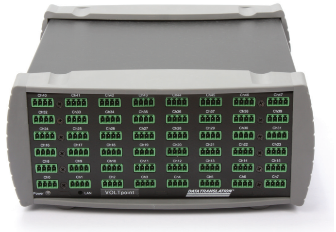
Figure 1. VOLTpoint allows direct battery cell connection of voltages up to \pm 400V with 1000V isolation between any of the 48 channels. Ground loops are eliminated through the isolation of each channel using the ISO-Channel technology.
