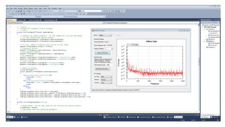
The Signal Processing Component Library for .NET is a comprehensive library of object-oriented classes ideal for developing signal processing applications. Each class contains properties and methods that can be used to perform single-channel and two-channel FFT operations, and to calculate signal metrics on time domain data. This library is included free with VIBbox.
