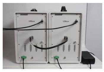
VIBboxes are connected together by attaching an EP377 Trigger Bus cable from the Sync Bus connector of one VIBbox to the Sync Bus connector of the next VIBbox. Each VIBbox must be powered using an external power supply and connected to a USB 3.0 port of a host computer.
