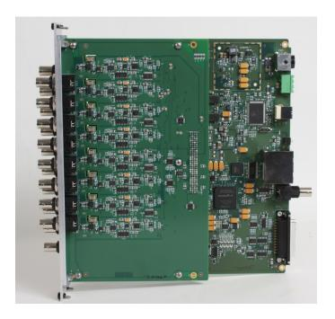
The DT9857E provides sixteen IEPE analog inputs, 2 analog outputs, 16 DIO, 1 counter/timer, 1 achometer, and 2 measure counters on each board set. VIBbox-64 packages four of these to bring the channel count to: 64 IEPE analog inputs, 8 analog outputs, 64 DIO, 4 counter/timer, 4 tachometers, and 8 measure counters. For more information on the DT9857E module, visit our web site: <a href="www.mccdaq.com/Products/Sound-Vibration-DAO/DT9857E">www.mccdaq.com/Products/Sound-Vibration-DAO/DT9857E</a>
